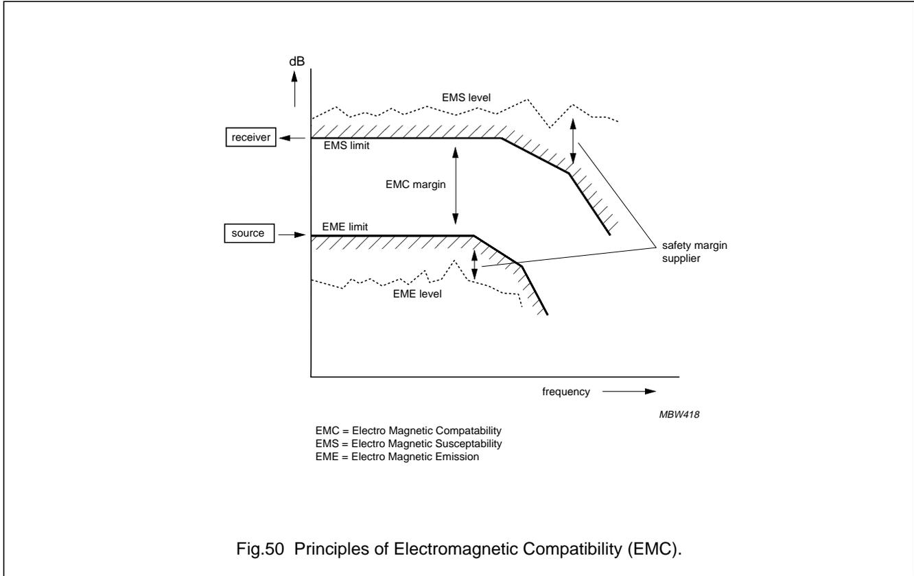
Fig.50 Principles of Electromagnetic Compatibility (EMC).
