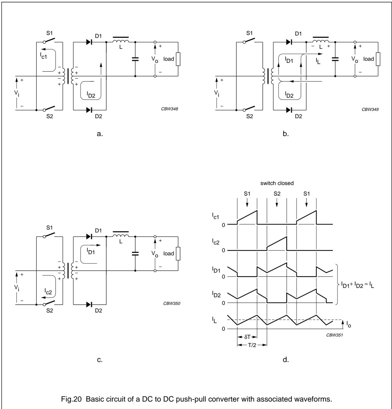
Fig.20 Basic circuit of a DC to DC push-pull converter with associated waveforms.
