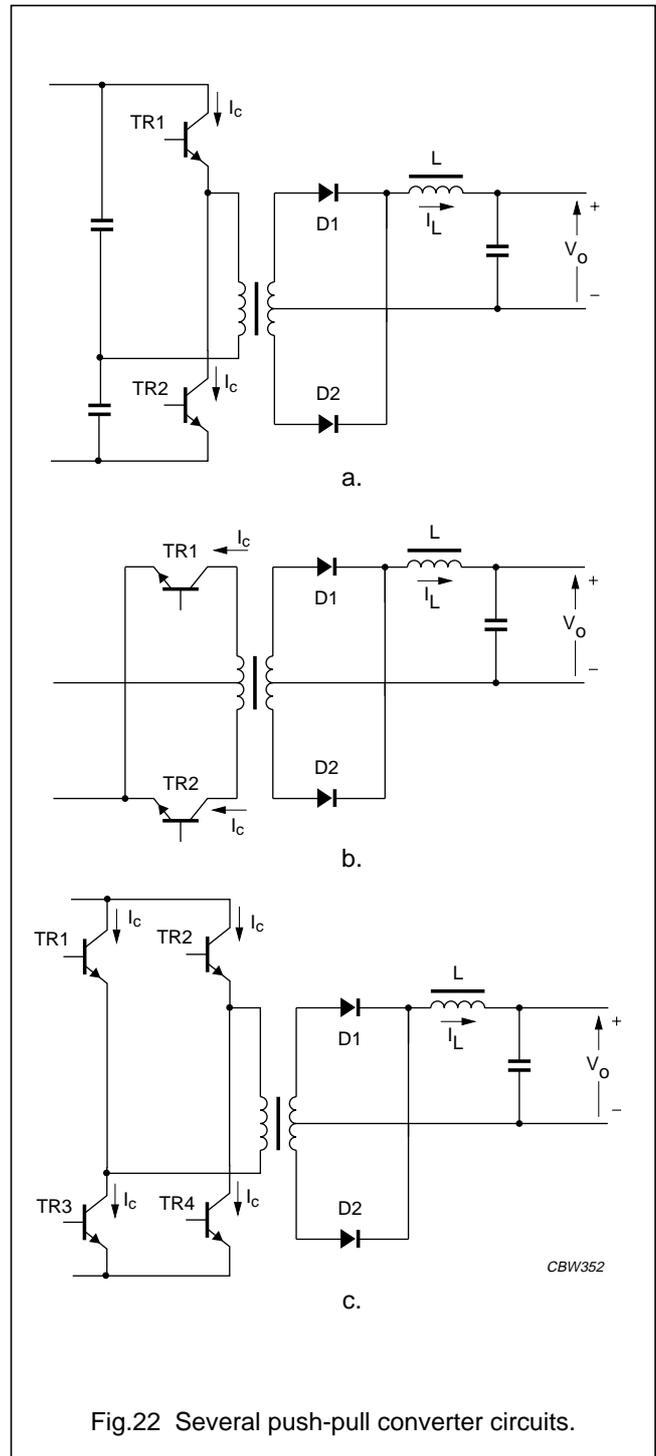
Fig.22 Several push-pull converter circuits.
