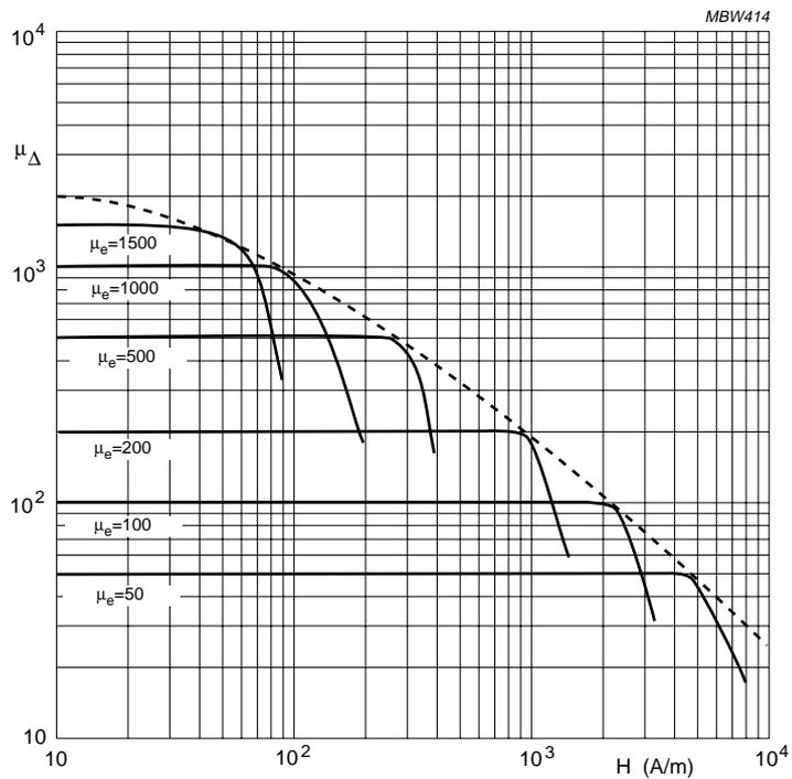
Fig.26 Effect of increased gap length.
