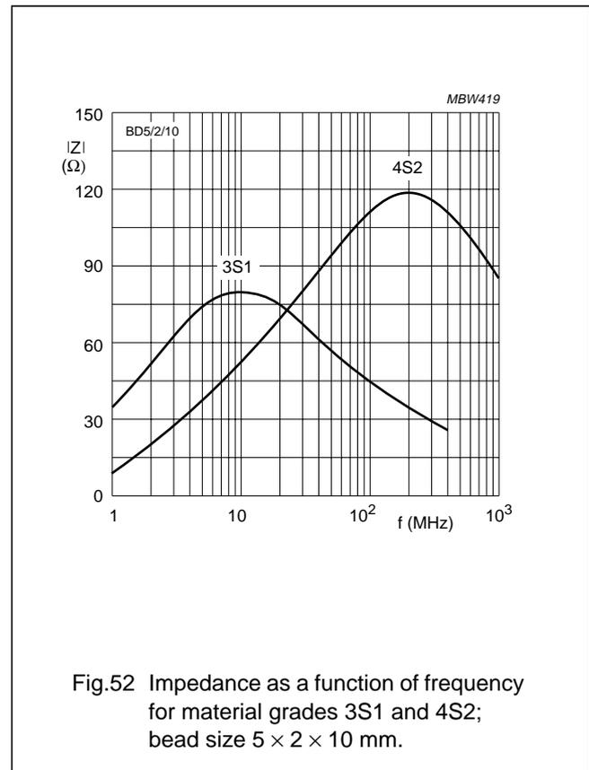
Fig.52 Impedance as a function of frequency for material grades 3S1 and 4S2; bead size  $5 \times 2 \times 10$  mm.
