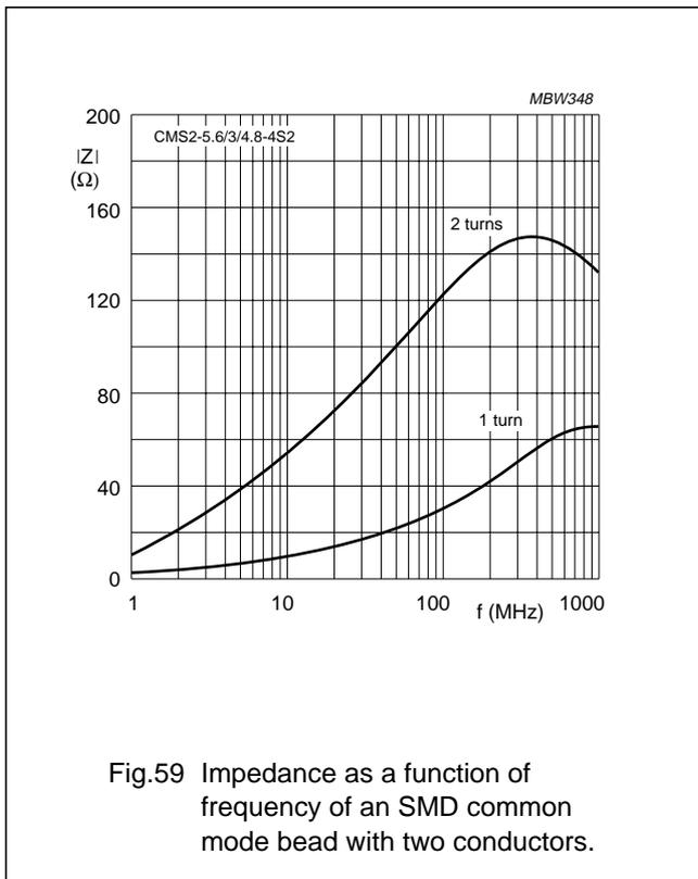
Fig.59 Impedance as a function of frequency of an SMD common mode bead with two conductors.
