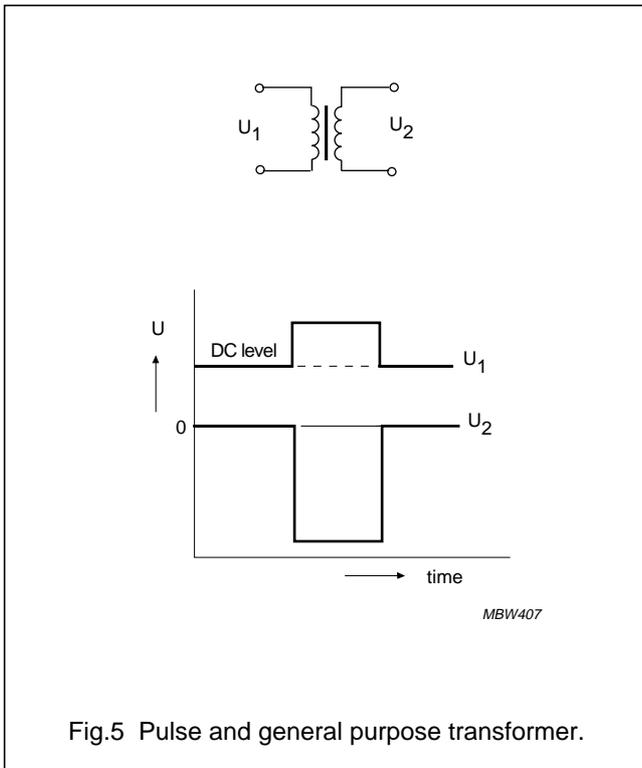
Fig.5 Pulse and general purpose transformer.
