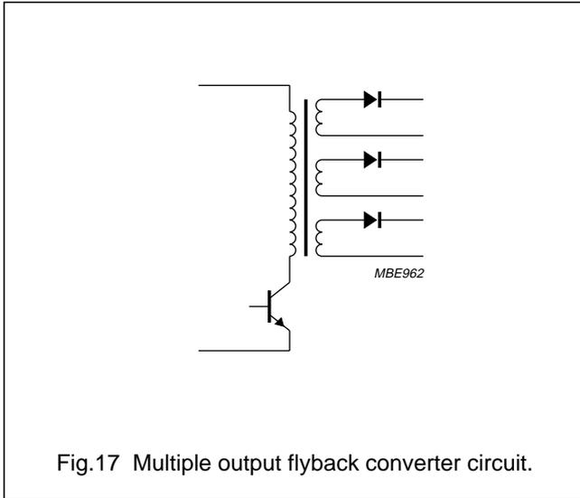
A disadvantage of this type of converter is that the output capacitor is charged only during the transistor's OFF cycle. Hence the output capacitor ripple current is high when compared with the other types of converters.
