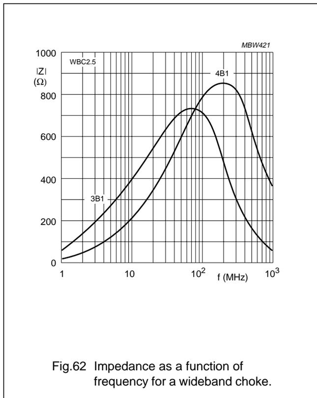
Fig.62 Impedance as a function of frequency for a wideband choke.
