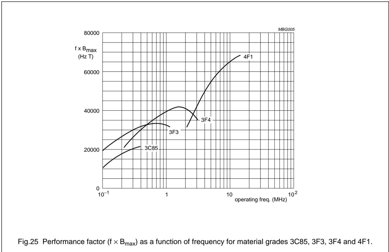
Fig.25 Performance factor ( $f \times B_{max}$ ) as a function of frequency for material grades 3C85, 3F3, 3F4 and 4F1.
