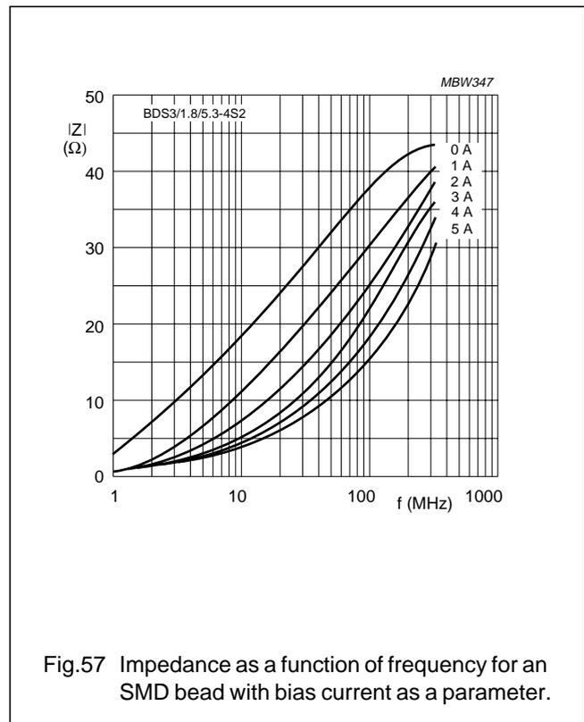
Fig.57 Impedance as a function of frequency for an SMD bead with bias current as a parameter.
