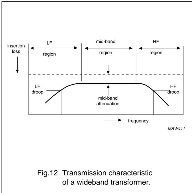
Fig.12 Transmission characteristic of a wideband transformer.
