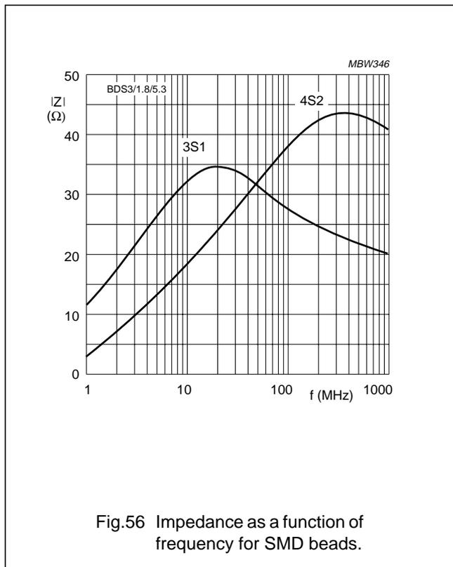
Fig.56 Impedance as a function of frequency for SMD beads.
