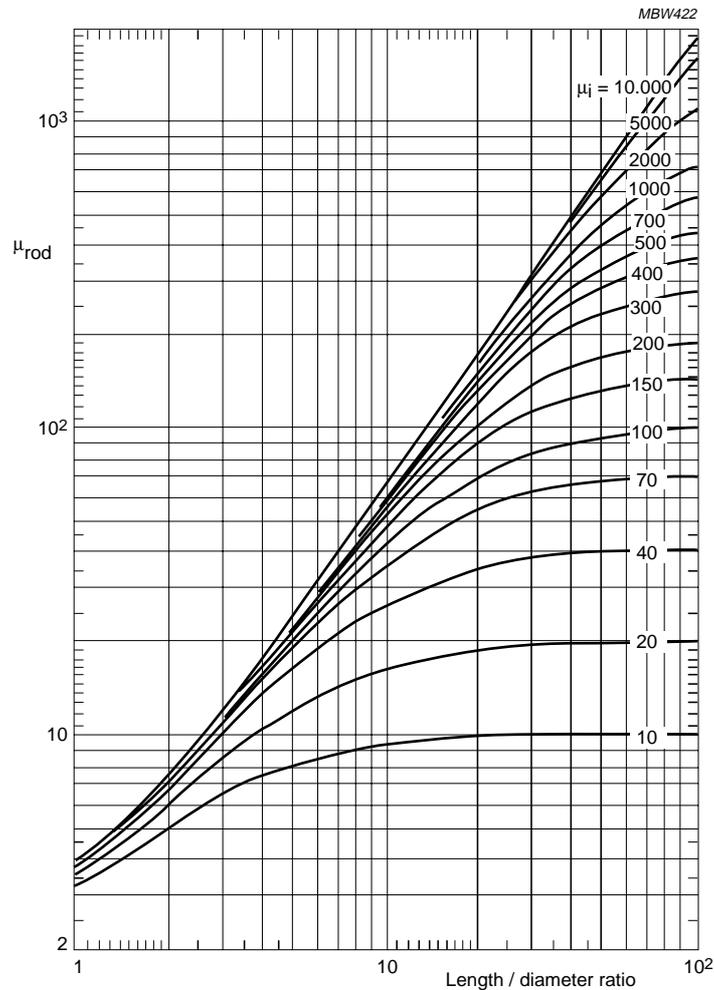
Fig.69 Rod permeability ( $\mu_{rod}$ ) as a function of length to diameter ratio with material permeability as a parameter.
