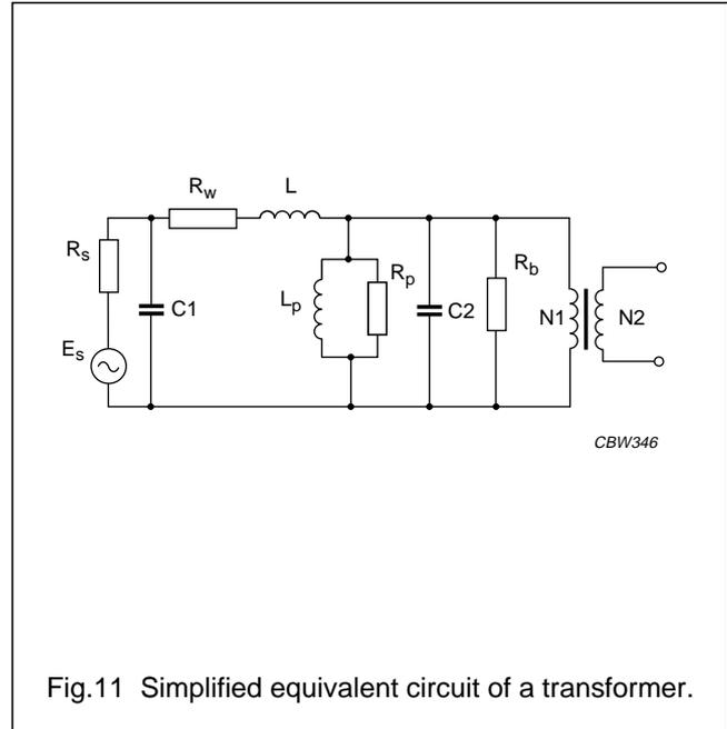
Fig.11 Simplified equivalent circuit of a transformer.
