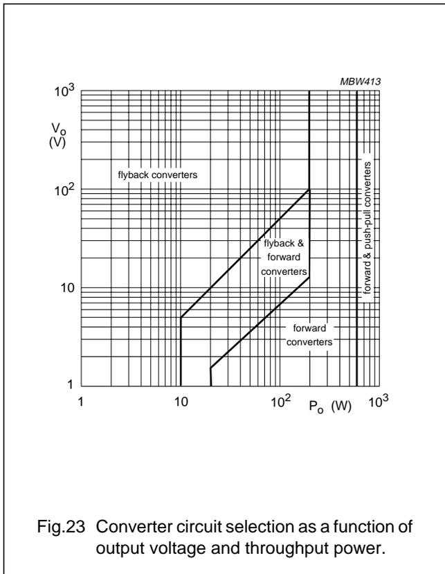
Fig.23 Converter circuit selection as a function of output voltage and throughput power.
