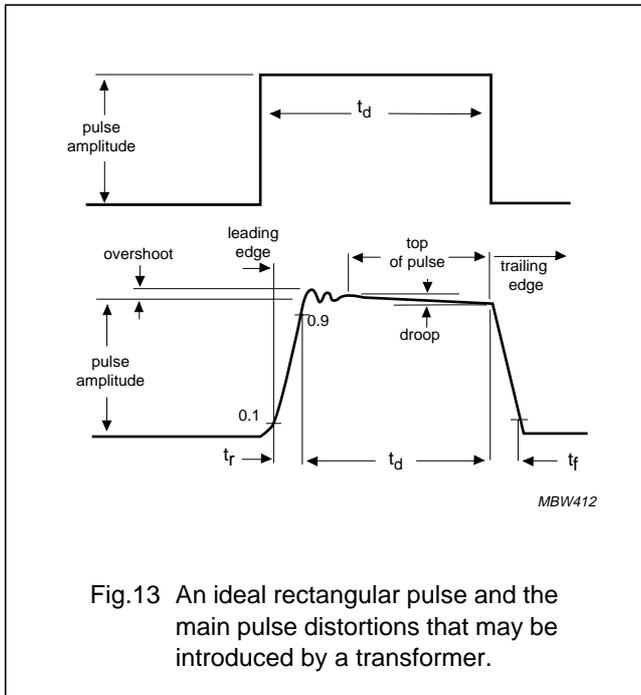
The shunt inductance ( $L_p$ ) is responsible for the low frequency droop in the analog transformer since its reactance progressively shunts the circuit as the frequency decreases. In the case of the pulse transformer, the shunt inductance causes the top of the pulse to droop, because, during the pulse, the magnetizing current in  $L_p$  rises approximately linearly with time causing an increasing voltage drop across the source resistance.
