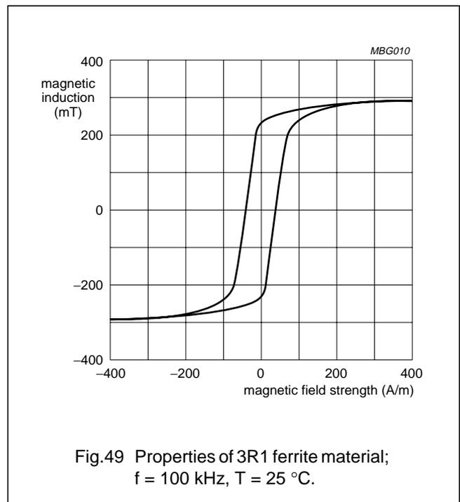
Fig.49 Properties of 3R1 ferrite material;  $f = 100 \text{ kHz}$ ,  $T = 25 \text{ }^\circ\text{C}$ .
