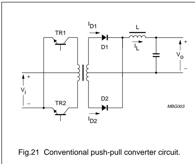
Fig.21 Conventional push-pull converter circuit.
