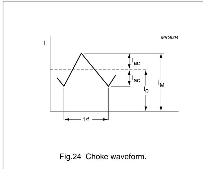
Fig.24 Choke waveform.
