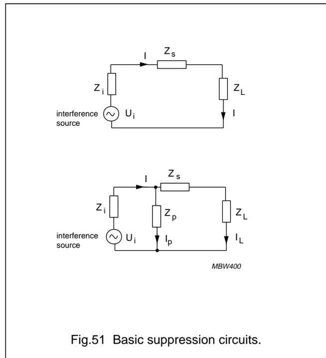
Fig.51 Basic suppression circuits.
