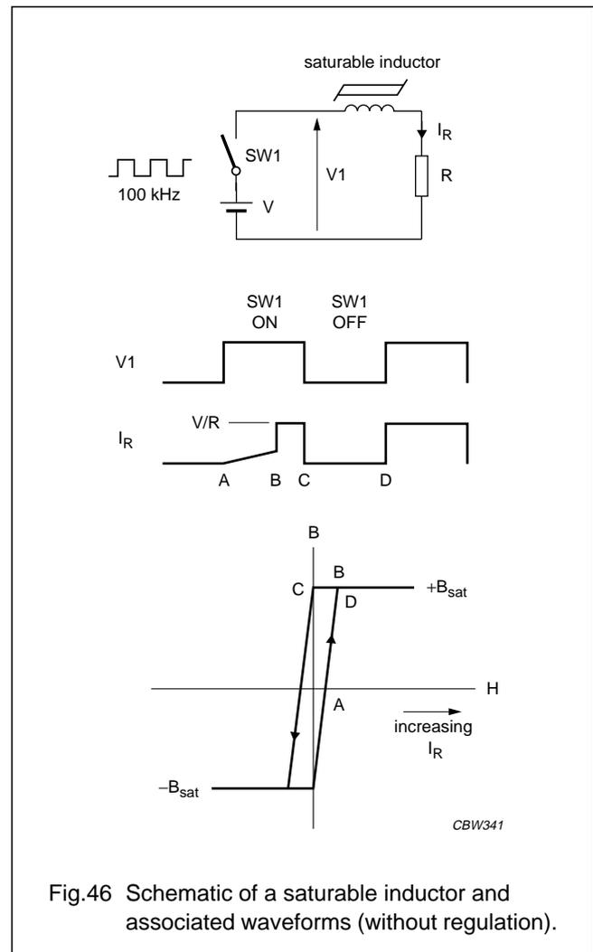
Fig.46 Schematic of a saturable inductor and associated waveforms (without regulation).
