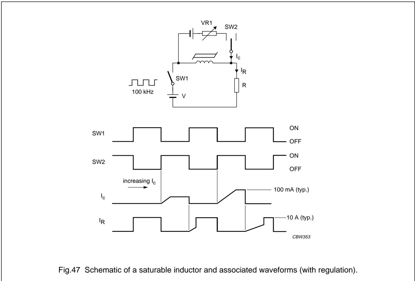
Fig.47 Schematic of a saturable inductor and associated waveforms (with regulation).
