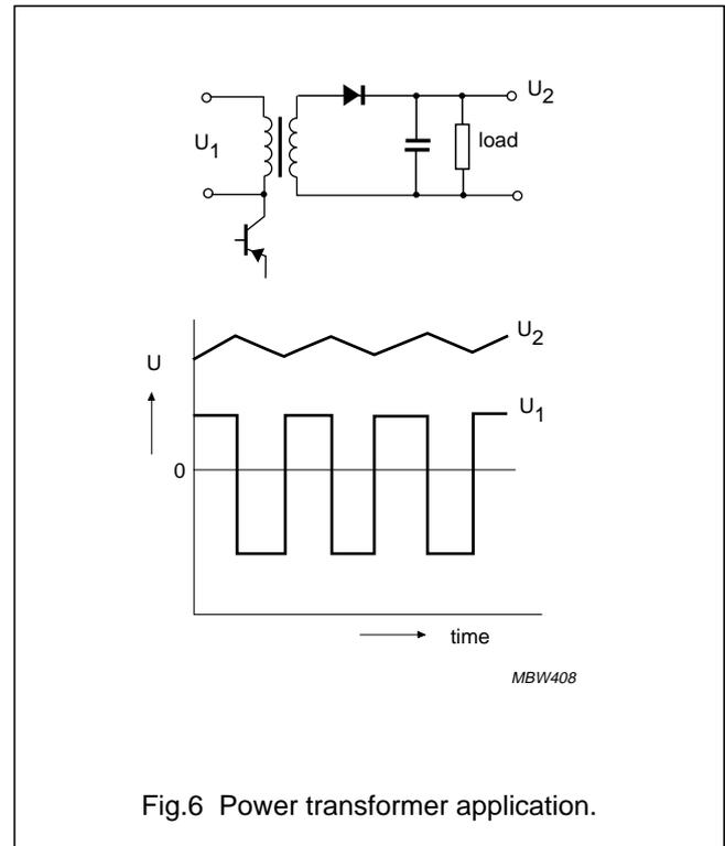
Fig.6 Power transformer application.
