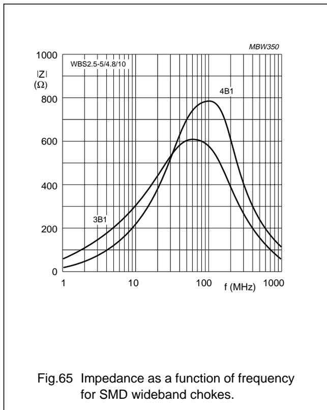
Fig.65 Impedance as a function of frequency for SMD wideband chokes.
