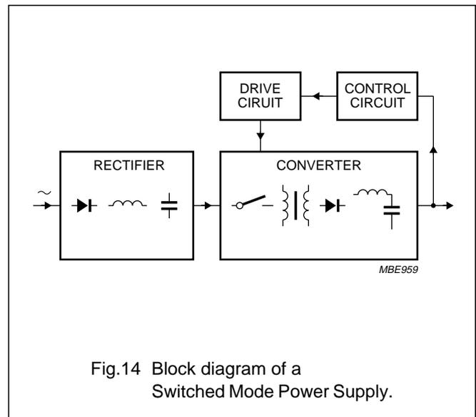
Fig.14 Block diagram of a Switched Mode Power Supply.
