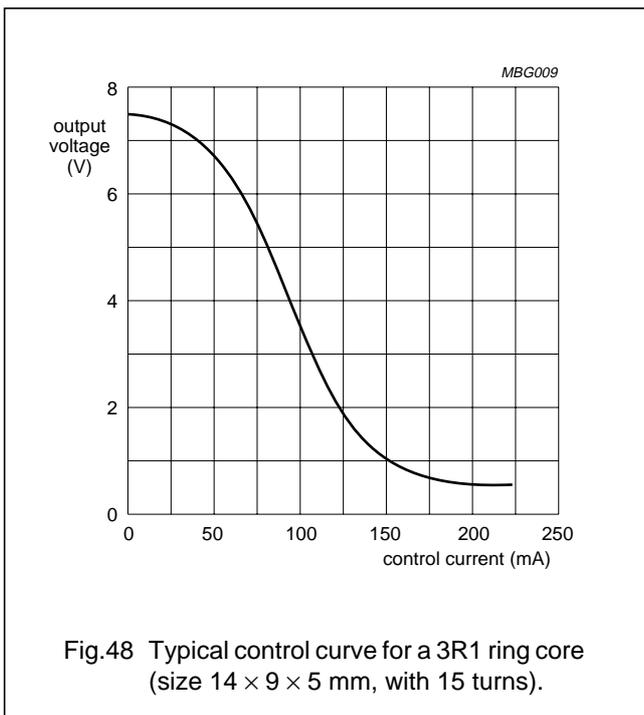
Fig.48 Typical control curve for a 3R1 ring core (size 14 × 9 × 5 mm, with 15 turns).
