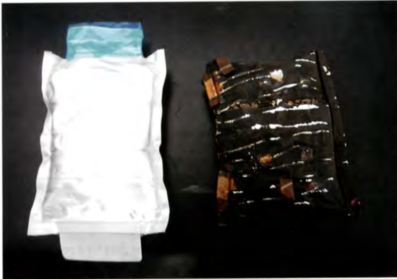
Figure 6 Li-ion Pouch battery before and after Thermal stability Test in adiabatic BTC
