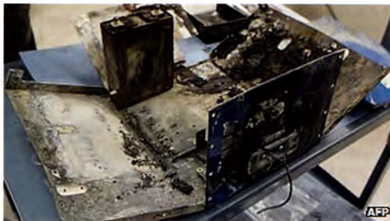
Figure 1 Photograph of Boeing Dreamliner Battery Enclosure after Fire
