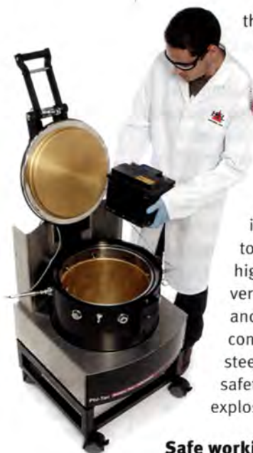
Figure 4 Custom designed adiabatic Battery Testing Calorimeter (BTC) for larger scale testing
