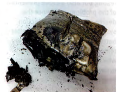
Figure 11 Li-ion NMC-graphite battery after Overcharging to 5V in adiabatic BTC
