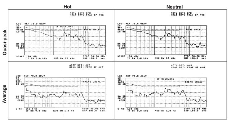
120VAC/60Hz Limits per 47CFR15.107 for Class B devices. 50mA total load.
