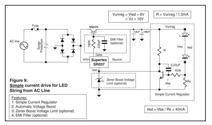
The circuit uses the SR037 or SR036 and GN2470 to drive a string of LEDs from AC power line.
