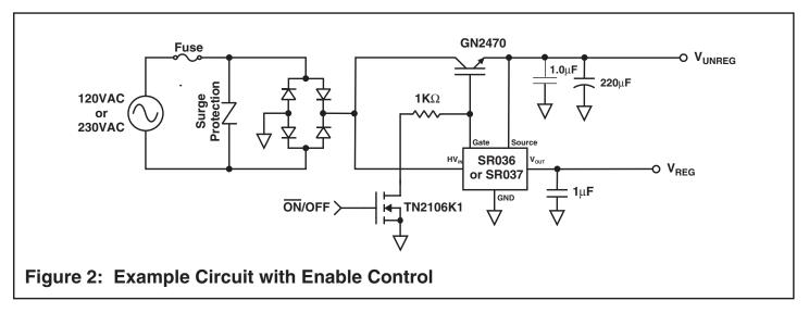
Figure 2 is an example circuit using the SR036 or SR037 along with a Supertex GN2470 IGBT to generate an unregulated voltage of approximately 18V and a regulated voltage of 3.3V for the SR036 or 5.0V for the SR037. The combined total output
