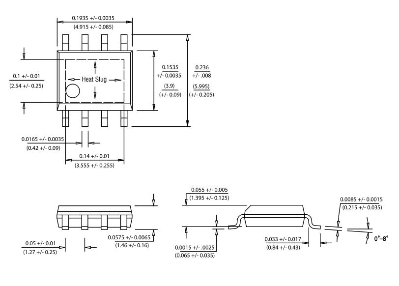
**Dimensions in Inches** Measurement Legend = (Dimensions in Millimeters)
