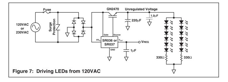
The circuit shown in Figure 7 uses the SR036 or SR037 to drive 12 high efficiency red LEDs from an AC line. The average LED current is approximately 20mA.
