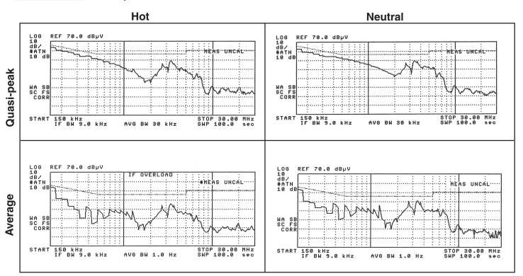
120VAC/60Hz Limits per 47CFR15.107 for Class B devices. 100mA total load.
