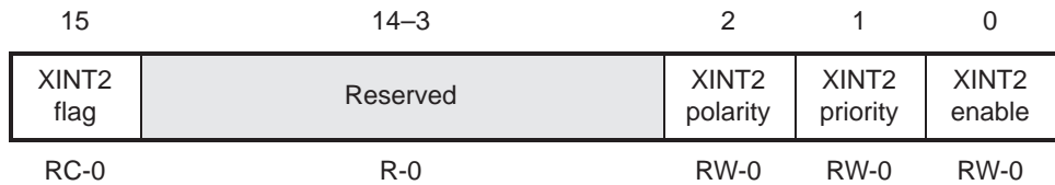
Figure 5–4. External Interrupt 2 Control Register (XINT2CR) — Address 7071h
