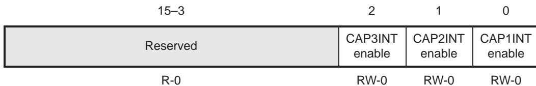
Figure 7–35. EV2 Interrupt Mask Register C — Address 742Eh
