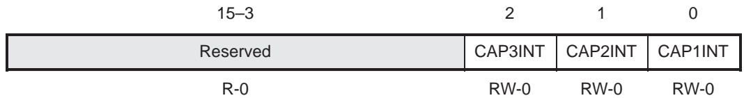
Figure 7–32. EV2 Interrupt Flag Register C (EVIFRC) — Address 7431h
