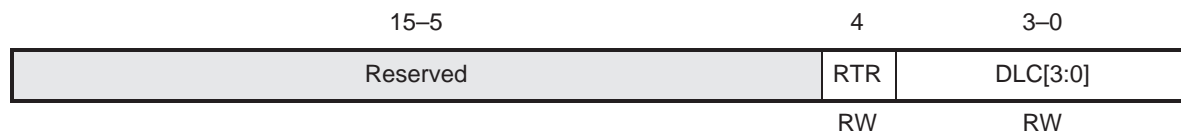
Figure 11–7. Message Control Field 0–5 (MSGCTRLn)
