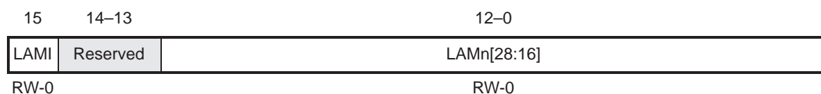
Figure 11–9. Local Acceptance Mask Register n (0, 1) High Word (LAMn_H)
