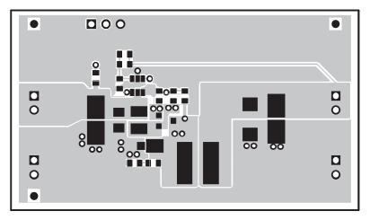
Figure 3–3. Bottom Layer Routing
