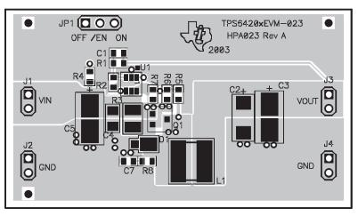
Figure 3–2. Top Layer Routing
