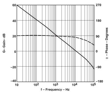
Figure 2–5. Overall Open Loop Response
