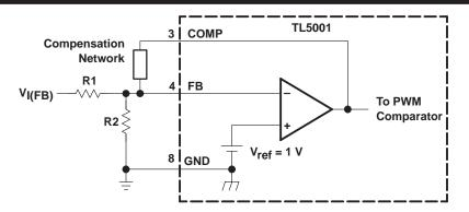
Figure 1. Error-Amplifier Gain Setting
