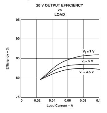
Figure 1–12. Efficiency vs Load 20-V Output
