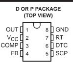
The TL5001 incorporates on a single monolithic chip all the functions required for a pulse-width-modulation (PWM) control circuit. Designed primarily for power-supply control, the TL5001 contains an error amplifier, a regulator, an oscillator, a PWM comparator with a dead-time-control input, undervoltage lockout (UVLO), short-circuit protection (SCP), and an open-collector output transistor.
