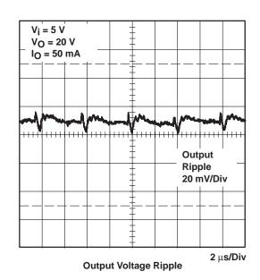
Figure 1–6. Output Voltage Ripple
