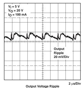
Figure 1–5. Output Voltage Ripple
