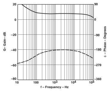
The overall open loop frequency response of the converter is the product of the uncompensated open loop response and the error amplifier response. A Bode plot of the overall open loop frequency response of the converter is shown below in Figure 2–5. The gain crosses 0 dB in the vicinity of 12 kHz and the phase margin is approximately 78 degrees.
