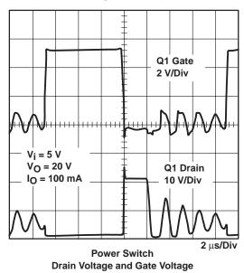
Figure 1–9. Power Switch Drain Voltage and Gate Voltage
