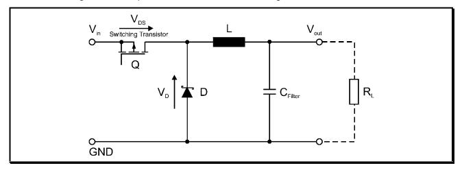
Figure 2.1: Schematic diagram of a Step-Down Converter
