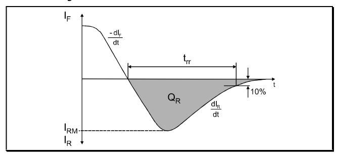
Figure 2.3: Switching behavior of a diode
