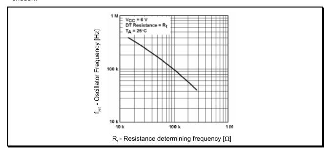
Figure 7.1: Oscillator frequency as a function of resistor  $R_t$
