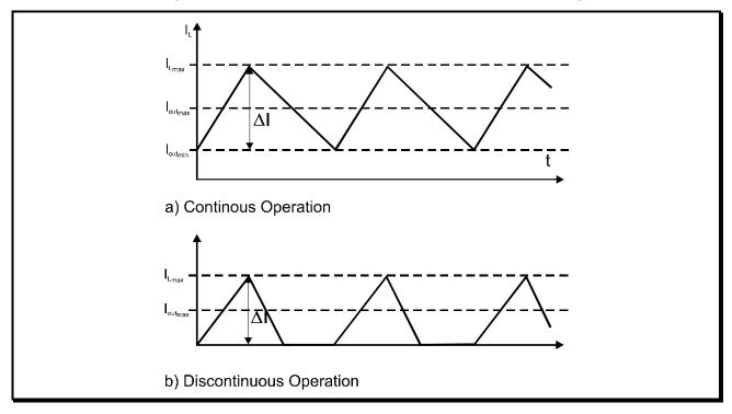
Figure 2.2: Inductor current, with continuous and discontinuous operation
