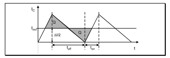
Figure 2.4: Curve of current in the capacitor
