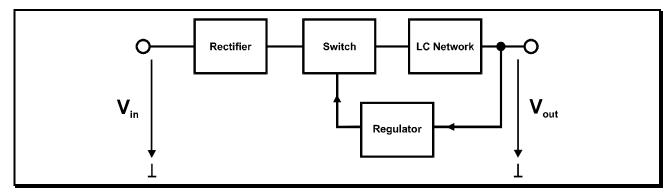
Figure 1.1: Block diagram of a Switched Mode Power Supply
