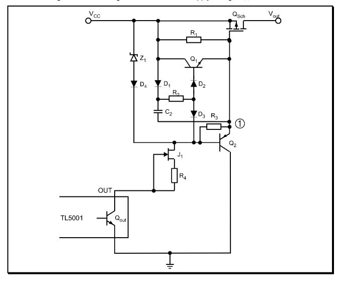
Figure 4.1: Limiting the Gate-Source voltage
