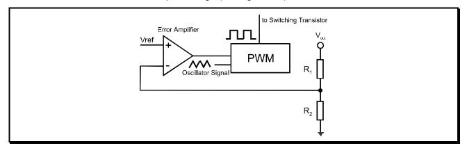
Figure 5.1: Schematic diagram of a pulse width modulator
