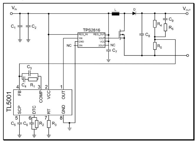
Figure 10.1: Step-Up Converter with the TL5001
