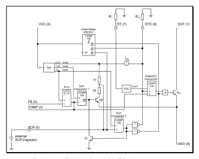
Figure 6.1: Functional diagram of the TL5001
