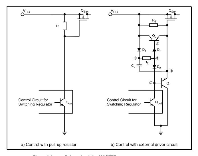
Figure 3.1: Driver circuit for MOSFET
