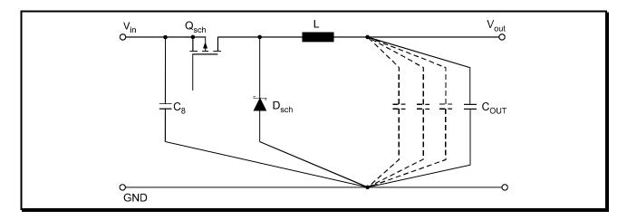
Figure 9.1: Layout for switching regulators
