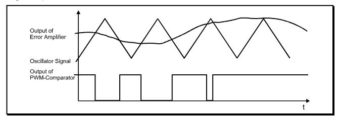
Figure 5.2: Principle of Pulse Width Modulation
