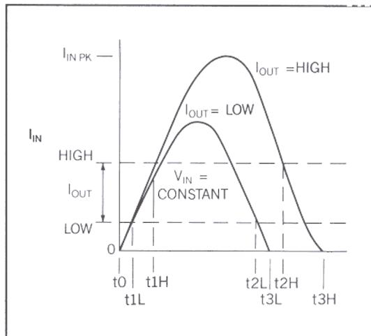
Fig. 15 - Effects of Load Change on  $I_{in}$
