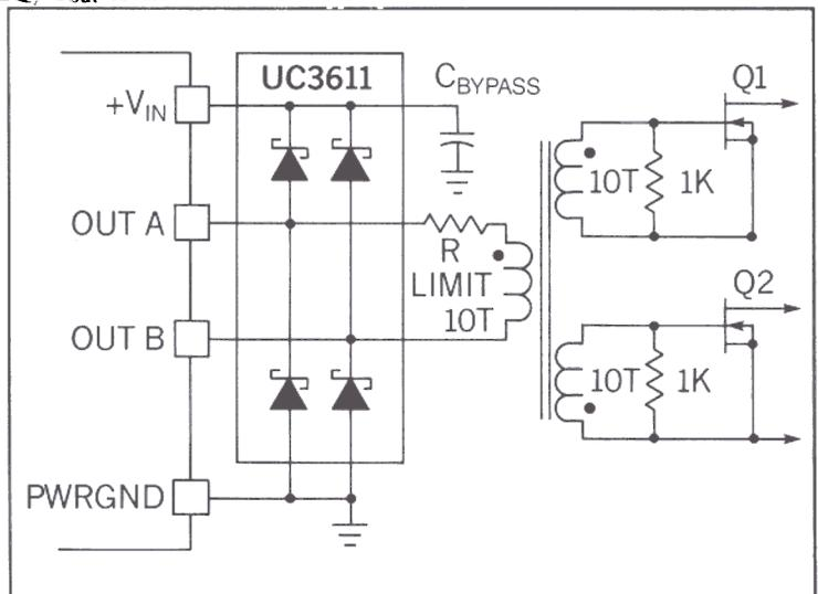
Fig. 23 - Gate Drive Circuit
