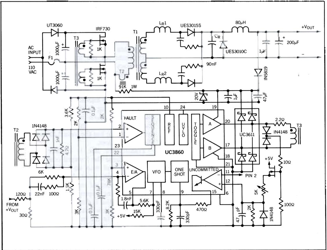
Fig. 3 - 150 Watt Off-Line Quasi-Resonant Half Bridge
