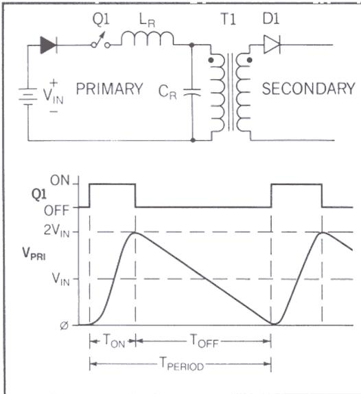
Fig. 6 - Primary Side Half Wave Resonance
