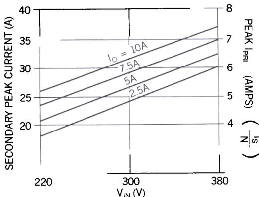
Fig. 16 - Peak Secondary Current vs.  $V_{in}$  and  $I_o$
