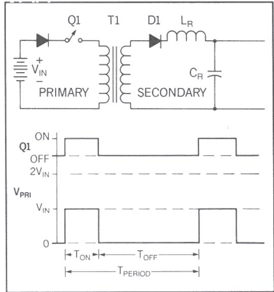
Fig. 7 - Secondary Side Half Wave Resonance
