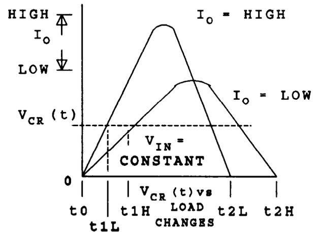
Fig. 8 -- Resonant Capacitor Voltage vs. Load to maintain a constant output current  $I_O$ . Its reverse voltage is clamped to the output voltage  $V_O$  minus the diode voltage drop  $V_{DO}$  by the convention followed by Figure 4.
