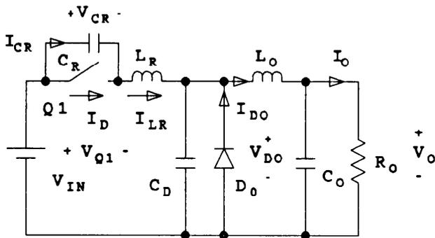
Fig. 21 -- Multiresonant ZVS Circuit
