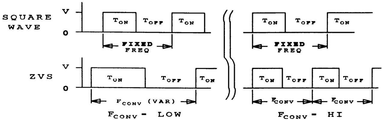
Fig. 1 - Zero Voltage Switching vs. Conventional Square Wave
