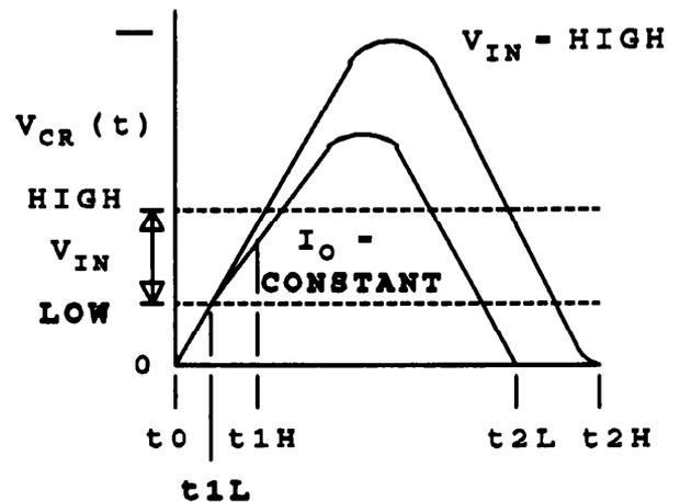
Fig. 7 -- Resonant Capacitor Voltage vs. Line
