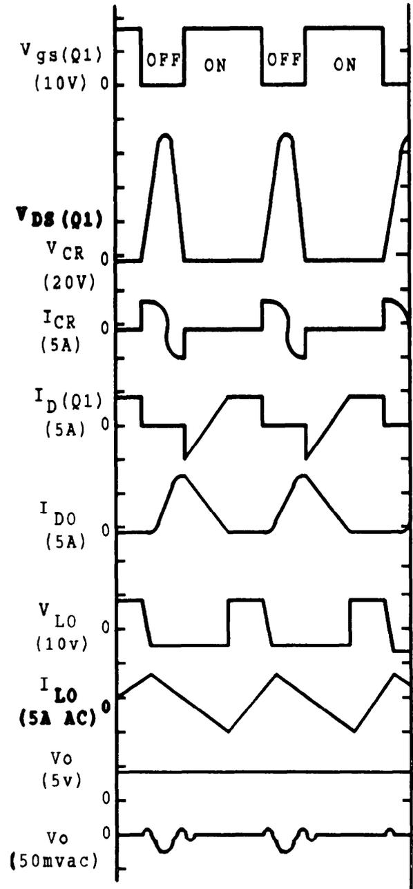
**ZVS Clamped Configurations -- Half and Full Bridge Topologies:** Zero voltage switching can be extended to multiple switch topologies for higher power levels, specifically the half and full bridge configurations. While the basic operation of each time interval remains similar, there is a difference in the resonant  $t_{12}$  interval.
