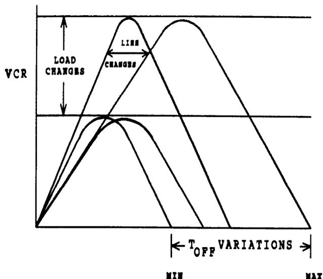
Fig. 26 --  $C_R$  Volts & Off-time vs. Line & Load
