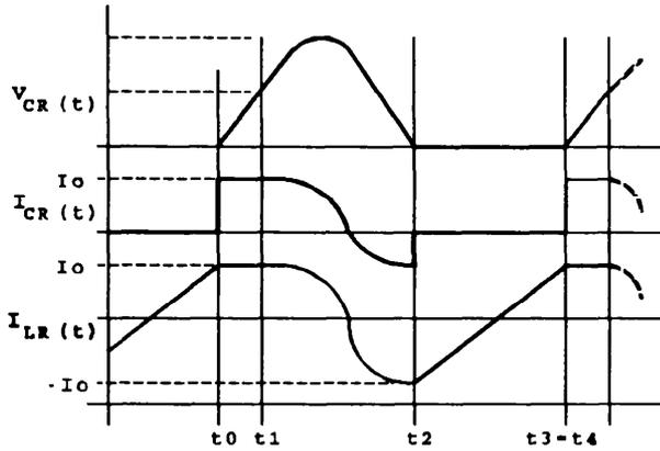
Fig. 10 -- Waveforms at  $F_{CONV} = K_T \cdot f_R$
