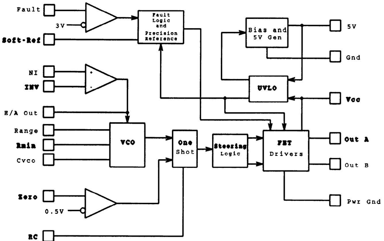
Fig. 25 -- The UC3861-64 ZVS Controllers -- Block Diagram
