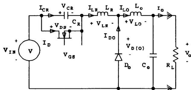
**Fig. 4 - Zero Voltage Switched Buck Regulator**
