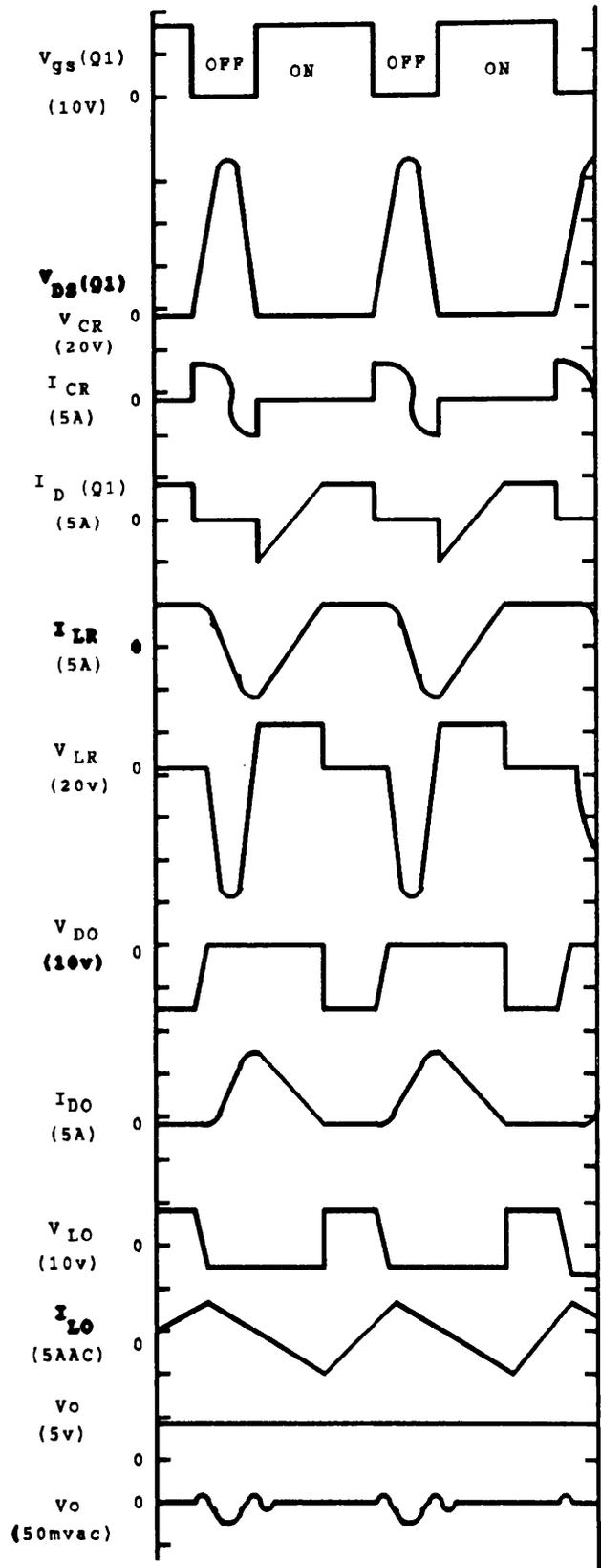
Fig. 9 -- ZVS Buck Regulator Waveforms
