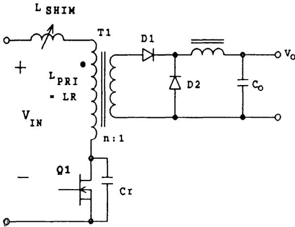
Fig. 12 -- ZVS Forward Converter
