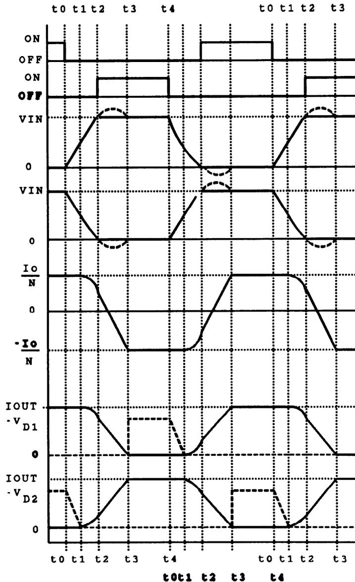
Fig. 19 -- ZVS Full Bridge Waveforms
