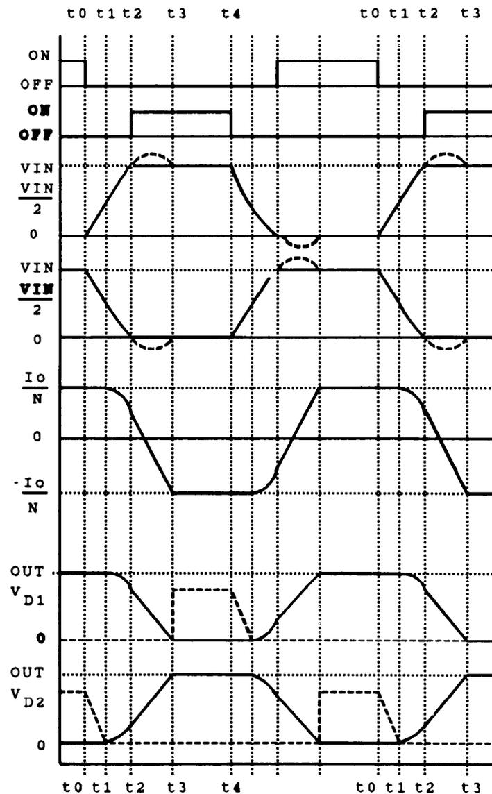
Fig. 17 -- ZVS Half Bridge Waveforms
