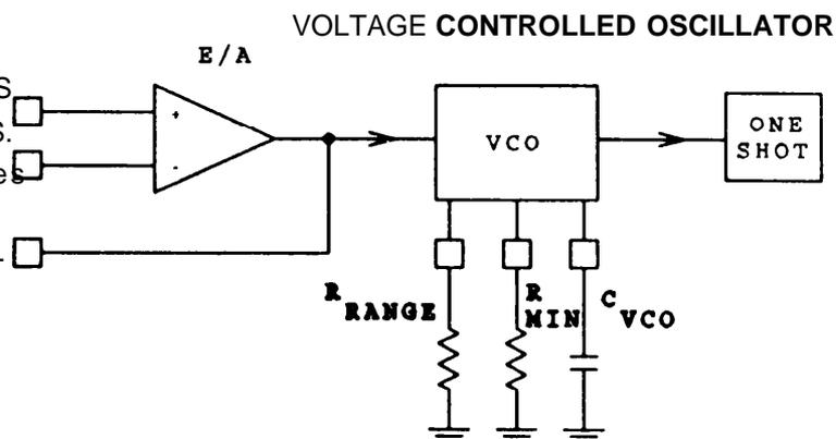
Fig. 27 -- E/A - VCO Block Diagram
