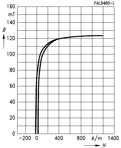
Dynamic magnetization curves (typical values) ( f = 10 kHz, T = 100 °C)
