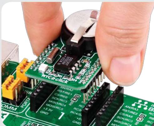
Once you have soldered the headers your board is ready to be placed into desired mikroBUS™ socket. Make sure to align the cut in the lower-right part of the board with the markings on the silkscreen at the mikroBUS™ socket. If all the pins are aligned correctly, push the board all the way into the socket.
