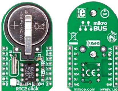
RTC2 Click is an accessory board in **mikroBUS™** form factor. It features the **DS1307** serial real-time clock (RTC). It is a low-power, full binary-coded decimal (BCD) clock/calendar with programmable square-wave output signal. Board uses I<sup>2</sup>C interface for communication, and can only use **5V** power supply. Board features a 3V/230mA **lithium battery** as a backup power supply which ensures that timekeeping operation continues even when the main power supply goes OFF.
