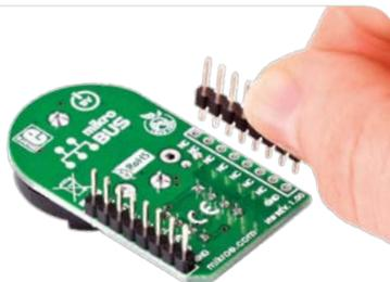
Turn the board upside down, so that bottom side is facing you upwards. Place shorter parts of the header pins in the both soldering pad locations.
