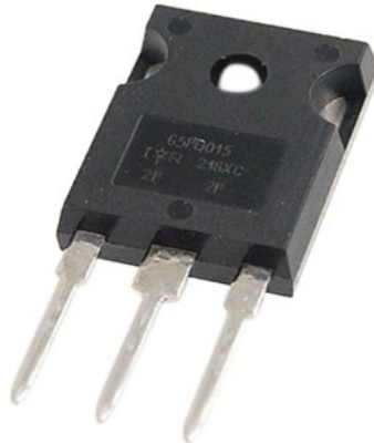
Illustration 15: Diode schottky T0-247AC 3
