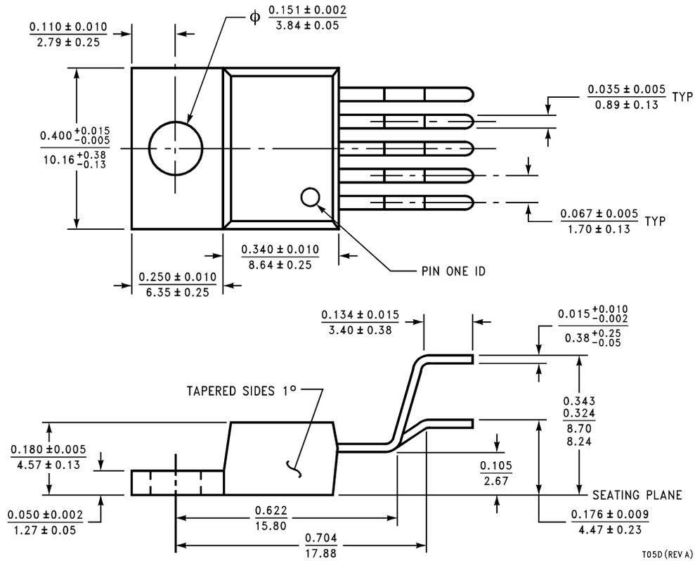
**5-Lead TO-220 Bent and Staggered Package**
