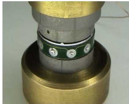
Fig. 3: Optimised piezo motor (M. Fluckiger PhD)
