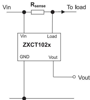
Figure 19 shows how a single sense resistor is required to measure current.
