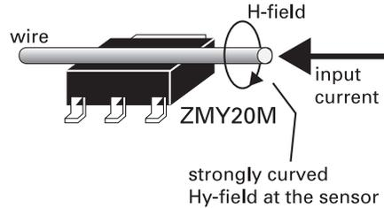
Figure 27 Internal cross-section of ZMC products
