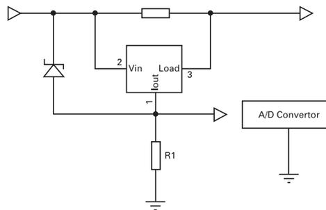
This will keep the ZXCT1009 within its permissible operating voltage by conducting at its zener voltage. R1 is used as normal to scale an appropriate output voltage.
