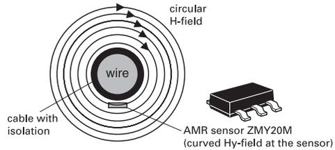
Figure 26 Sensing small diameter cables
