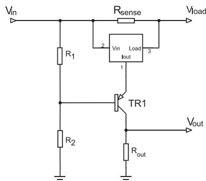
TR1 is used in common base configuration and is used to drop most of the supply voltage between collector and emitter. When the current gain is reasonably high ( $>100$ ),  $I_C \approx I_E$  and  $I_{out}$  still flows through  $R_{out}$  and hence  $V_{out}$  can be calculated in the normal way.
