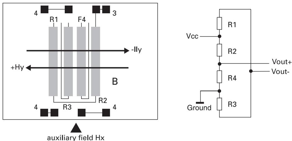
4.21 Sensor position for external conductors
