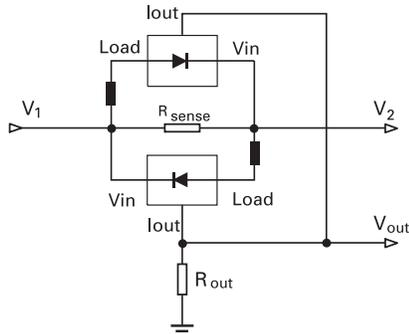
Non-linearity will be apparent at small values of  $V_{SENSE}$  due to offset current contribution, therefore the ZXCT1010 would be preferred to minimise this. Devices can use separate output resistors if the current direction is to be monitored independently.
