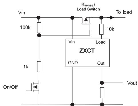
**Figure 23 Measuring forward and reverse currents separately**
