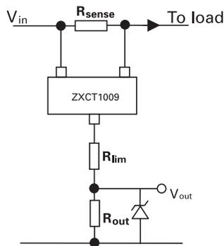
Assuming the worst case condition of  $V_{out} = 0V$ ; providing a low impedance to a transient, the minimum value of  $R_{lim}$  is given by:-
