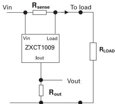
Figure 8 shows the basic configuration for monitoring a current.  $R_{LOAD}$  represents any load, such as a DC motor, charging battery or any other circuit which requires a current monitor.
