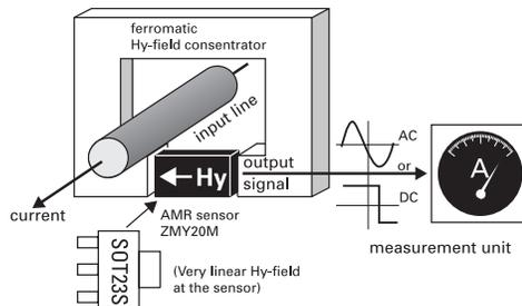
A core of ferromagnetic material, for example iron for mains frequencies, can be used to enclose all the lines of flux from a conductor which has the following properties:
