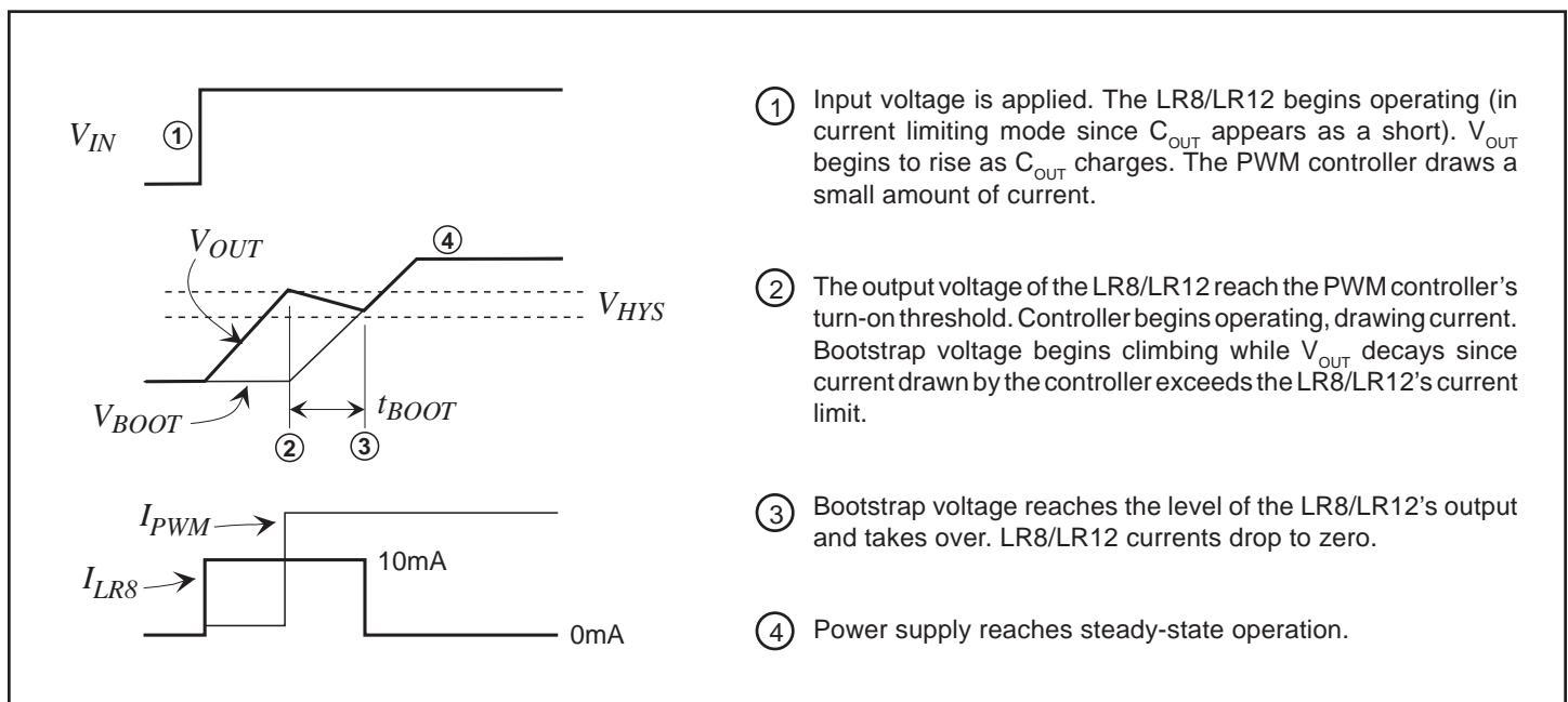
The minimum capacitance required for given boot-up time is given by the following equation:
