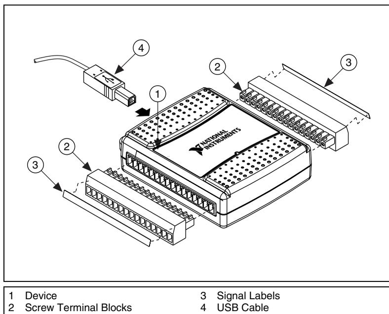
The USB-6008/6009/6501 ships with signal labels. You can apply the signal labels to the screw terminal blocks for easy signal identification. Select the signal label best suited for your application. Refer to the user guide for your device for more information about signal names.
