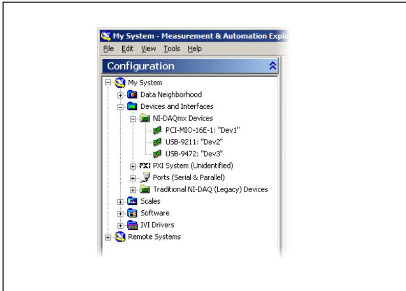
3. Check that your device appears under Devices and Interfaces. If your device does not appear, press <F5> to refresh the view in MAX. If the device is still not recognized, refer to [ni.com/support/install](http://ni.com/support/install) for troubleshooting information.
