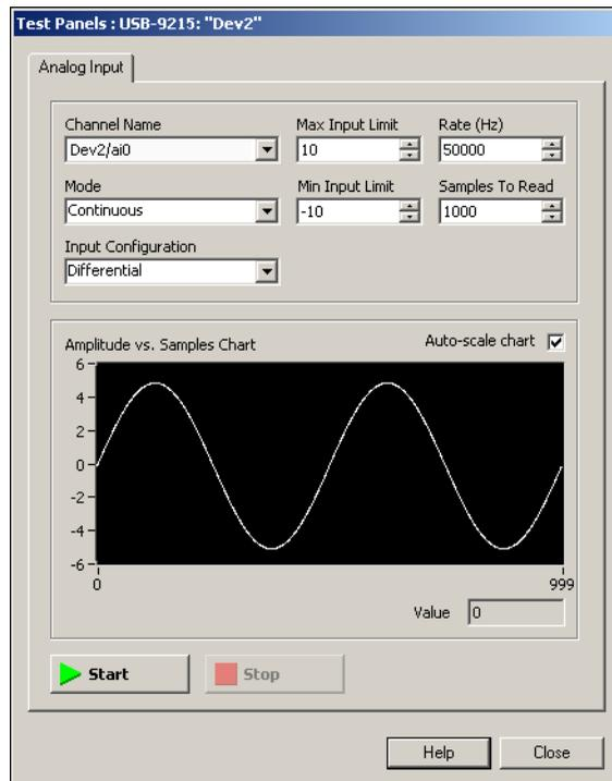
4. Click **Start** to test different functions of the device. Click **Help** for instructions on operating the test panels.
